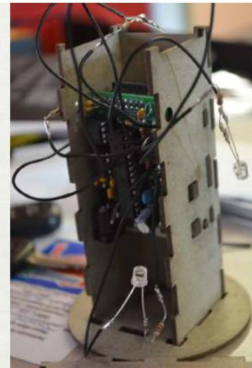
The mount is the external structure which encapsulates the jar and was designed to provide support for the construction. It was first modeled in Rhinoceros 3D which was then fabricated using a CNC router in four individual pieces with every piece having a different inner diameter length and angle. After fabrication, the pieces were glued together and manually sanded to perfection before final assembly.
